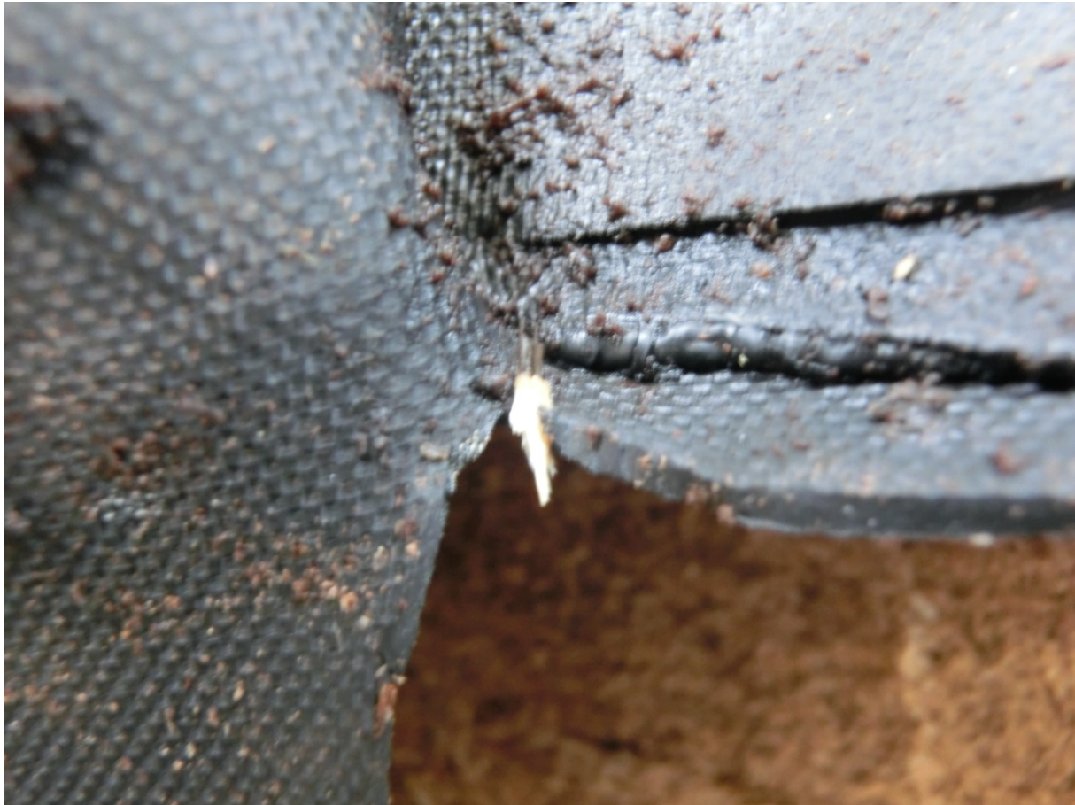
Figure 5: Perforation of the membrane by a rhizome (inner face of the membrane)
